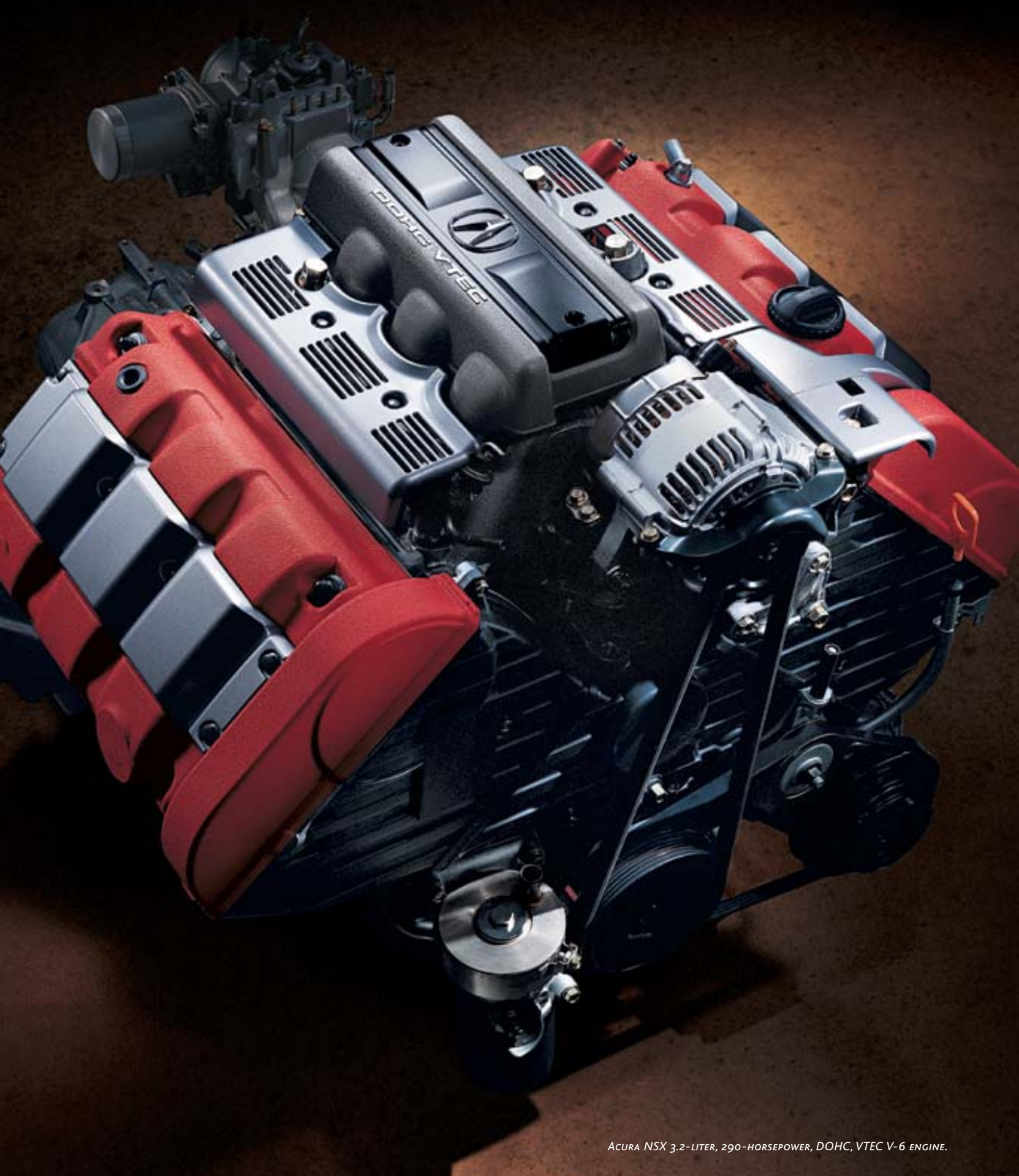
VTEC SPREADS THE POWER BAND BY SWITCHING BETWEEN TWO DISTINCT CAM PROFILES ON BOTH THE INTAKE AND EXHAUST CAMSHAFTS, VARIABLE VALVE TIMING AND LIFT ELECTRONIC CONTROL (VTEC) PROVIDES THE PERFECT AIR/FUEL AND EXHAUST FLOW CHARACTERISTICS FOR LOW-SPEED TORQUE AS WELL AS HIGH-RPM HORSEPOWER. THIS INNOVATIVE TECHNOLOGY WAS INTRODUCED TO THE U.S. ON THE FIRST NSX.
